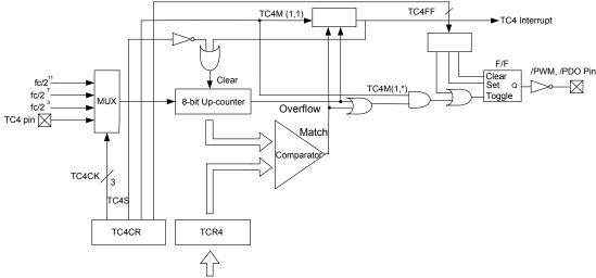
Fig. 25. Timer/Counter 4 Configuration
